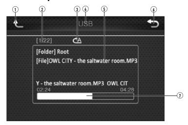
MP3/WMA/JPG Playback from Disc, USB Device or microSD Card To play MP3, WMA and JPG files from a disc, USB device or micro SD card. Insert disc, connect USB device or insert microSD card, and playback will begin automatically. To return to disc, USB or microSD card playback from another mode of operation, select the DISC, USB or SD icon from the Main Menu screen or top icon display, or press MODE until DISC, USB or SD is selected
